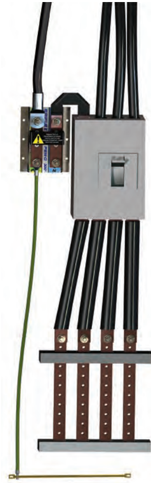
Dedicated TN-S Power Supply
